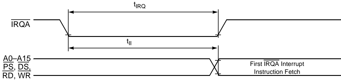
Figure 21. Recovery from Stop State Using \overline{\text{IRQA}} Interrupt Service
